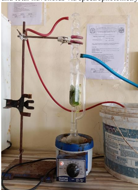
Figure 10. Preparation of Extract by using Soxhlett Apparatus.
